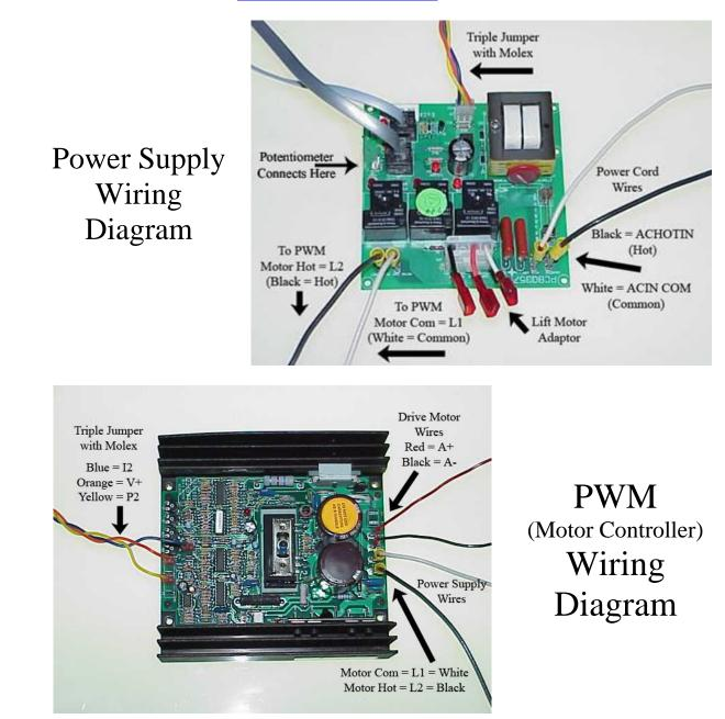
G. Refer to the Power Supply Diagram to check the connections as you plug in the two Lift Motor wires, the Power Cord wires, and the PWM power wires.
